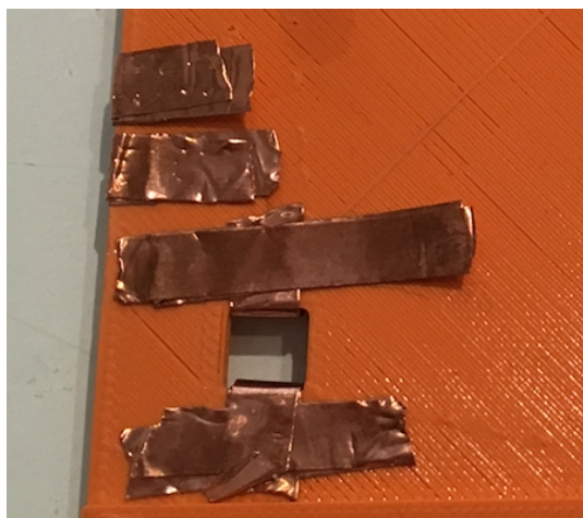
Figure 4: One of Carlotta's series of tests for developing a reliable copper tape button for Makey Makey.
