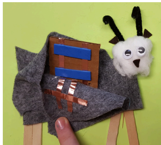
Figure 2: Copper tape button embedded in a crafted goat.
