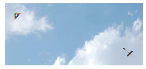
The Air Column Profiler Aeropod, being flown by a kite in the above photo, is used to capture a variety of atmospheric parameters throughout the air column.
